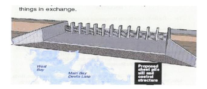
The Tolna Coulee Control Structure should never be operated under the U.S. Army Corps of Engineers original operating plan. The op. plan states, "Once stop logs are removed from the structure to allow discharge they will not be replaced for the purpose of holding water in Stump Lake." (p. 2)
