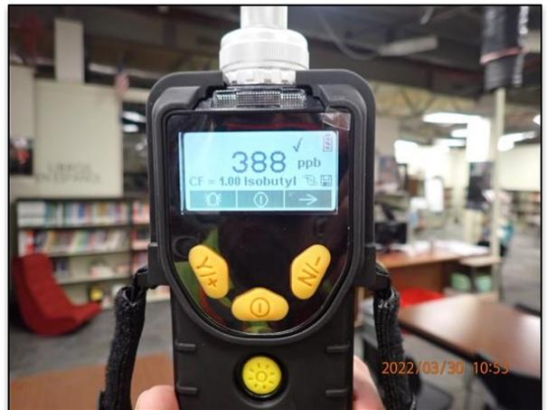
Figure (12) – PID Meter measurement of 388 parts per billion (ppb) library.
