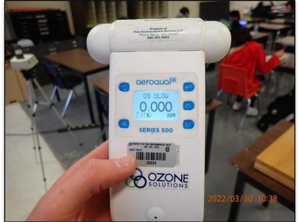
Figure (8) – Ozone monitor reading of 0.000 ppm in Room 3.
