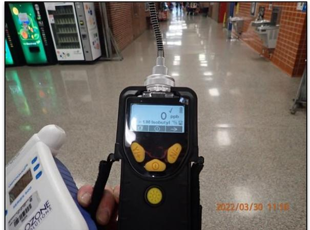
Figure (16) – PID meter reading of 0 ppb in corridor between main building and gymnasium building.
