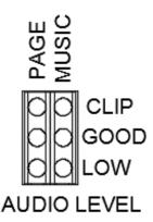
The Audio Level LEDs indicate the audio level input for the paging and music signals. Low (yellow) indicates a low audio level, Good (green) indicates a good audio level, and Clip (red) indicates an audio level that is too high, and clipping is occurring.
