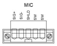
The microphone input is for a dynamic microphone.
