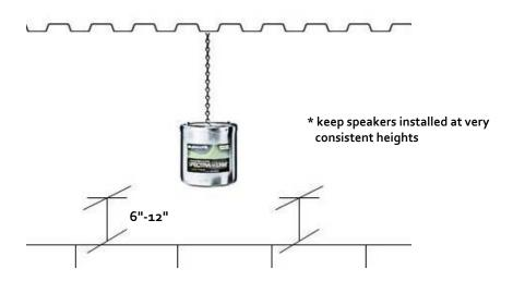
NOTE: If installing Inline speakers, make sure the potentiometer on the bottom of the speaker is set to the MAXIMUM (clockwise) setting.
