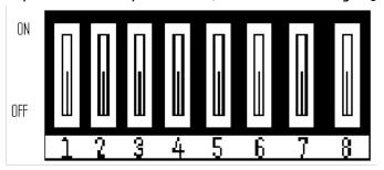
The IR Touch Pad Controller comes with all dip switches in the down position by default.
