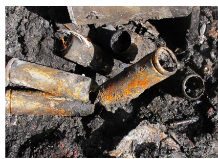
The remnants of the lithium battery that caught fire in Weston last month causing "a lot of damage."
