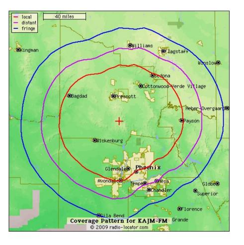
Effective Radiated Power 40,000 Watts Height above Avg. Terrain 807 meters (2649 ft) Height above Ground Level 52 meters (171 ft) Height above Sea Level 2323 meters (7626 ft) Antenna Pattern Non-Directional Full Class C, FCC Rated Station
